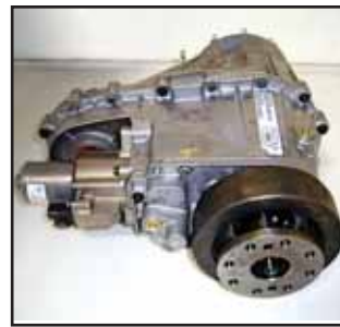
Rear of transfer case
