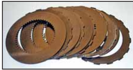
Steel side of clutch plates
