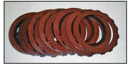
Lined side of clutch plates
