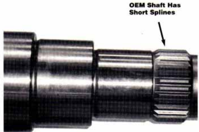
OEM shaft showing short spline length
