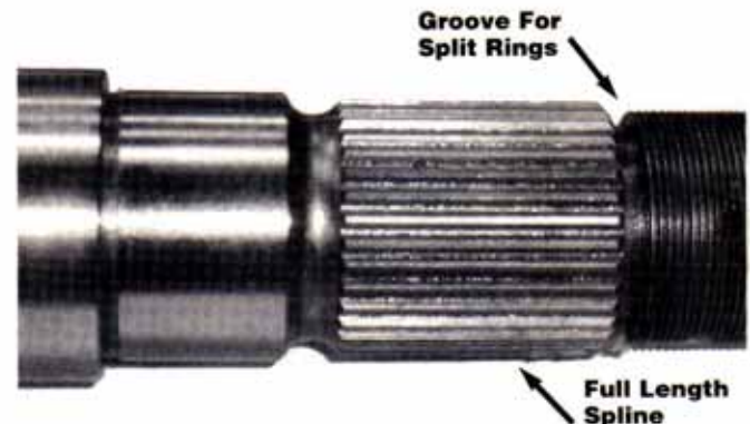
Aftermarket shaft with full length spline Groove for split rings
