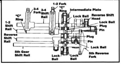
5. Reverse blockout also may occur because of worn shift components, bad clutch hydraulics, worn clutch assemblies, peened-over gear teeth because of poor clutch release, failure to wait for the clutch to spin down and reverse shifts attempted with the vehicle rolling forward.
